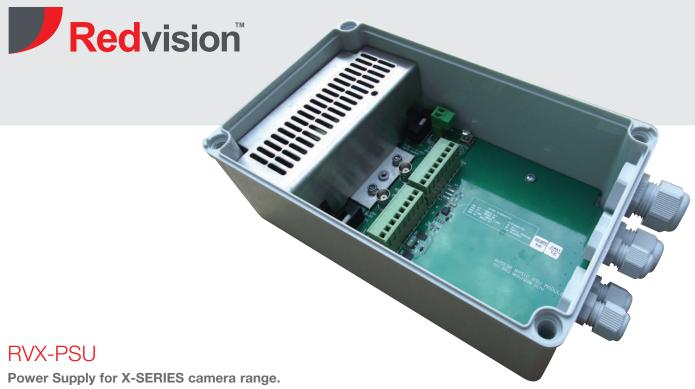
Connectivity to the X-SERIES camera and control equipment is made via pluggable terminal blocks. Video cable has option of terminal block or BNC connection. Weatherproof enclosure to IP 67 comes complete with range of cable glands ready fitted. Both 485 and video lines have lightening protection designed to protect the camera from high voltage spikes.
