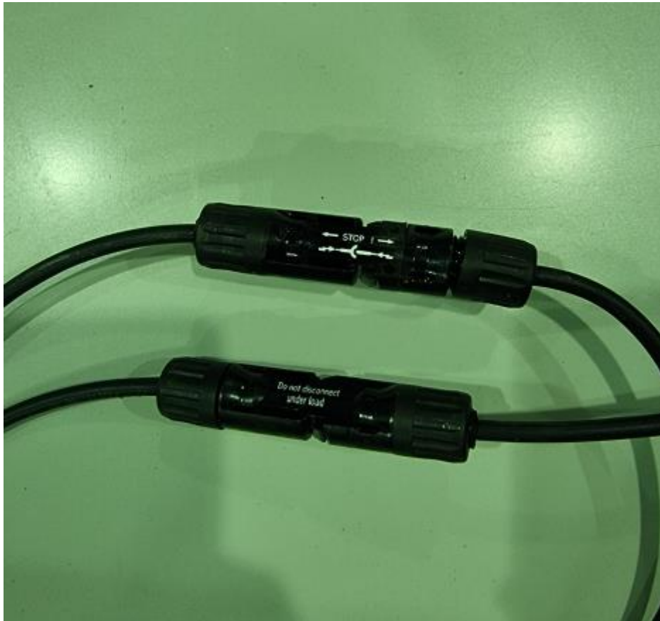
Figure 20: Connecting Solar Panel.
