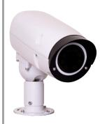
**VEGA-THERMAL-15-PED:** Fully cable managed camera housing and pedestal bracket. POE+, 12V DC, 24V AC. Factory fitted 640 x 512 resolution, ≤40mK Thermal Box Camera, 15mm fixed lens. Ruggedised marine finish.
