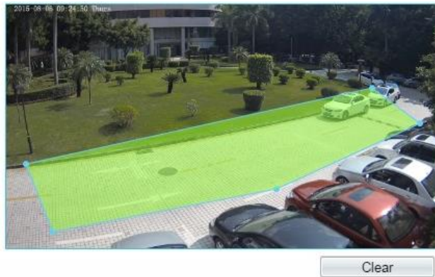
Figure 1-27 Deployment Area Setting Interface
