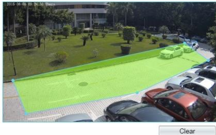
Figure 1-16 Deployment Area Setting Interface
