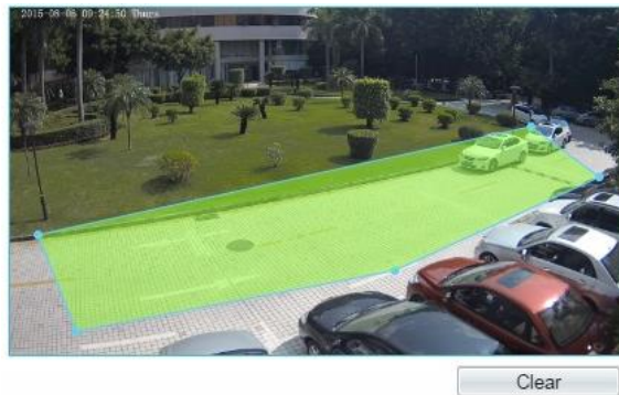
Figure 1-29 Deployment Area Setting Interface
