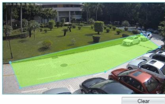
Figure 1-35 Deployment Area Setting Interface
