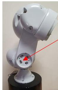
Slacken all Allen screws on each tilt-arm (4mm key), then move head gently forwards.
