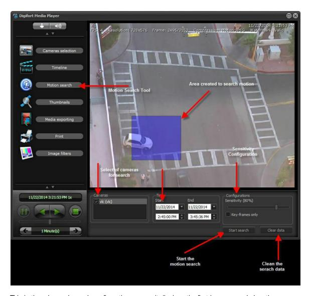
This is the advanced search configuration screen; it displays the first image recorded on the camera in the specified time interval, and provides the following features:
