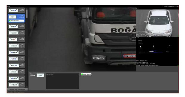
The screen central image shows the last plate recognized, or the plate selected in the event bar on the left.
