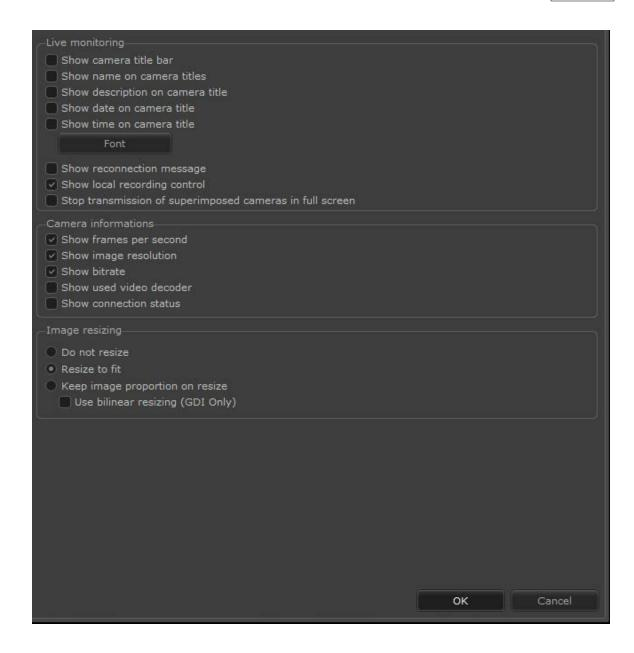
This configuration is divided into three parts: live surveillance configuration, camera information, and configuration of image resizing.
