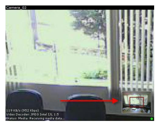
Once the zoom has started, all the Pan and Tilt options will be enabled. The Virtual Joystick can also be used with the Digital PTZ.
